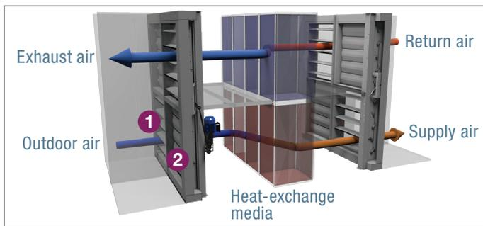
*Alternating dampers open or close every 20 seconds to charge or discharge energy in the heat-exchange media.*
