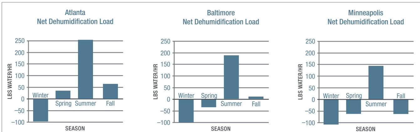
Data based on minimum 25% outdoor air, occupied mode
