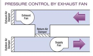
Using a centralized exhaust fan to control space air pressure is a preferred and common method for almost any space. Note that the exhaust fan shown here is in the air handling unit, but it may be located elsewhere.
