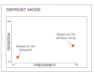
Triggering defrost based on only the ambient temperature may cause refrigeration circuits to go into defrost mode regardless of whether the outdoor coil is truly frosted or not. Using additional data from the unit, such as compressor suction pressure and outdoor air dewpoint, is the best way to determine when there is frost on the outdoor coil and defrost mode is therefore required.
